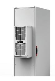
**Description:** SpectraCool with advanced corrosion system is the air conditioning solution for environments that are exposed to harsh, corrosive, chemical elements. Units have an active condensate management. Cleanable, reusable aluminium mesh filter protects coils for maximum cooling performance. The mechanical thermostat is inside the unit. The factory setting is 27 °C.
