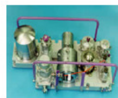
ARIANE 5 Main Stage Pressure Regulating Module
